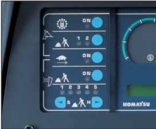
Track shoe slip control panel
